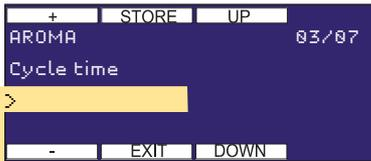
Defines the aroma cycle time (spraying time + spraying interval). Only active in systems without aquaCool or disabled aquaCool.
