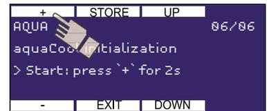
Starts the aquaCool initialization process. A spraying cycle of 90 seconds is started to bleed the system before commissioning, after a repair operation or after a canister replacement.
