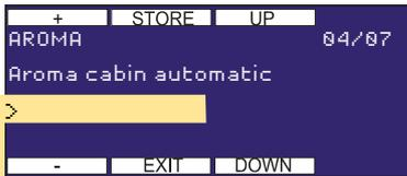
The cabinet scent release can be set at intervals, controlled by a door contact switch, or completely deactivated.
